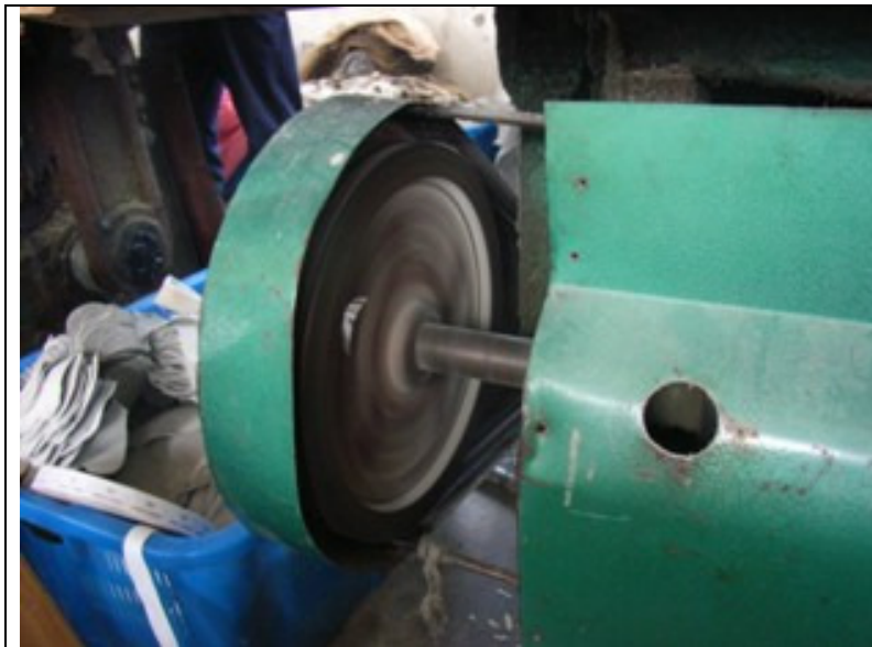
Safeguards on the punching machines
